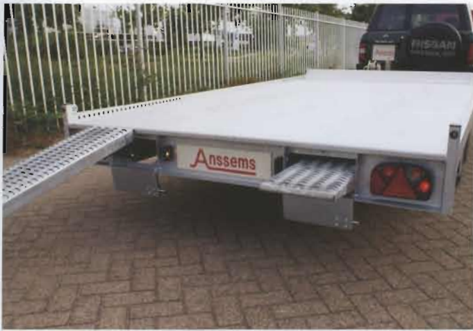
Ramps and rampstorage
